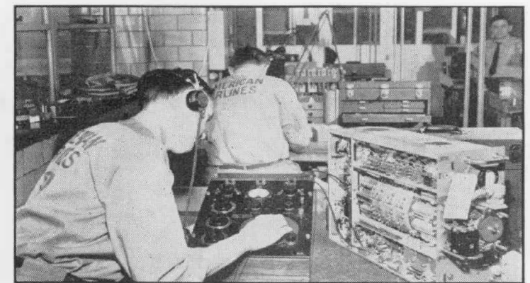
FIGURE 2. The TYPE 631-B Strobotac is used to check vibrator reeds by James Hargreaves, lead mechanic in radio-overhaul shop.
